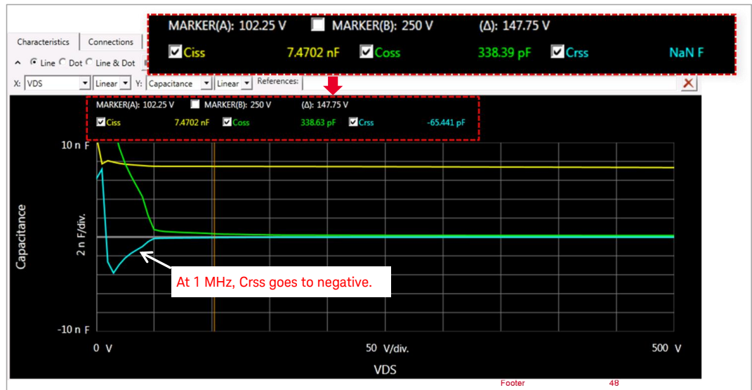
Figure 4-19 Crss measurement example (linear Capacitance scale) at 1 MHz (super junction FET).
